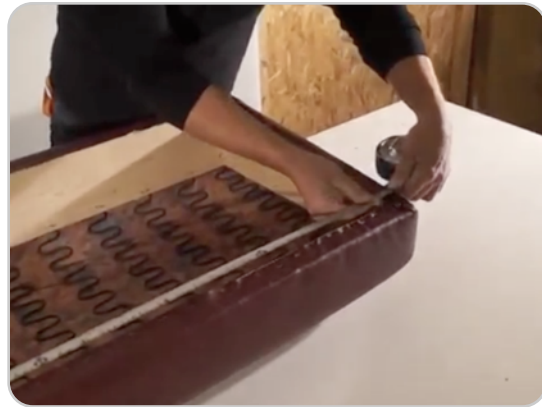
Step 2: With your seat upside-down, get your "A" measurement. (The entire length of the seat.)
